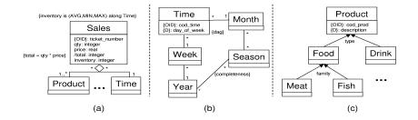
Fig. 1. Multidimensional modeling using the UML
