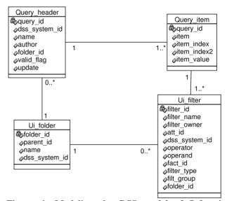
Figure 4: Modeling the DSS model of Informix Metacube (dynamic part) with UML
