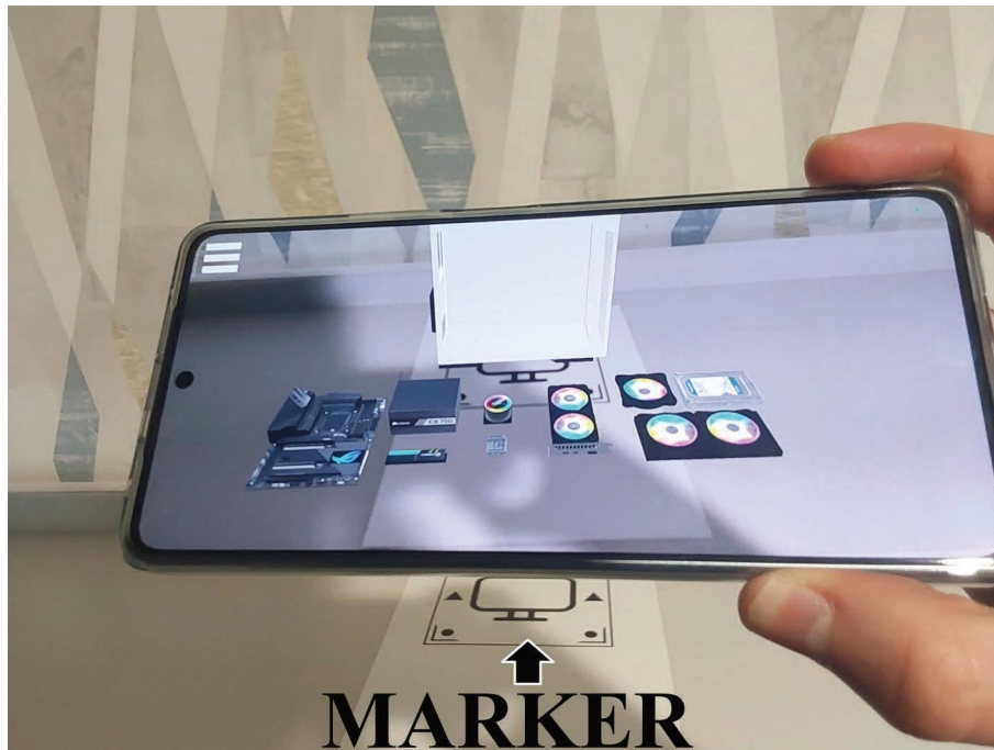
FIGURE 1 | Build_PC in operation, 3D elements are displayed over the real image captured by the mobile phone camera.
